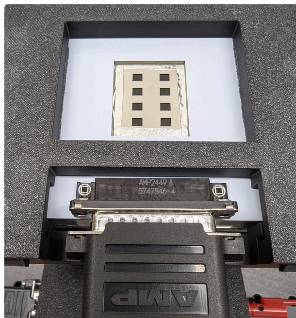
Figure 4: Cell in alignment jig
