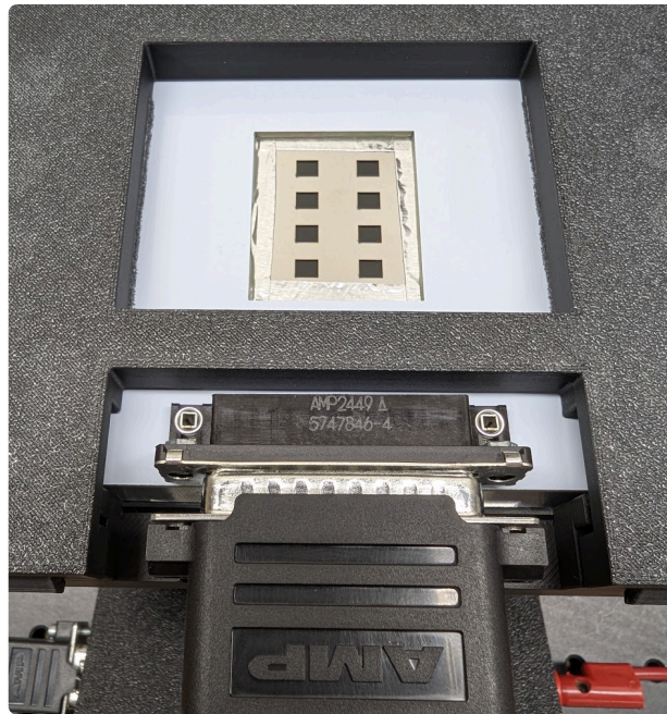
Figure 2: Cell in alignment jig
