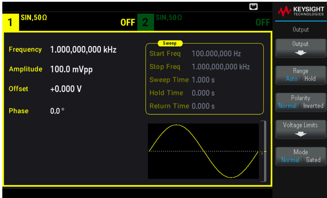
Figure 21: Keysight EDU33212A Setup Menu
