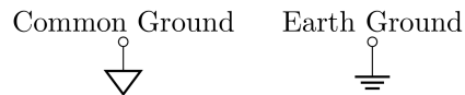
Figure 2: Common ground is a point at which you are arbitrarily calling 0 V. Earth ground is a connection to the Earth.
