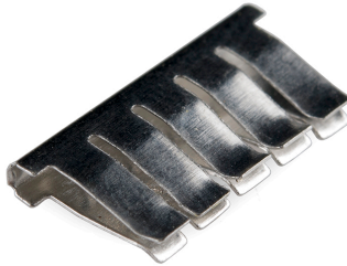
Figure 2: The breadboard is composed of many of these rows of grabbers. Image from Sparkfun.
