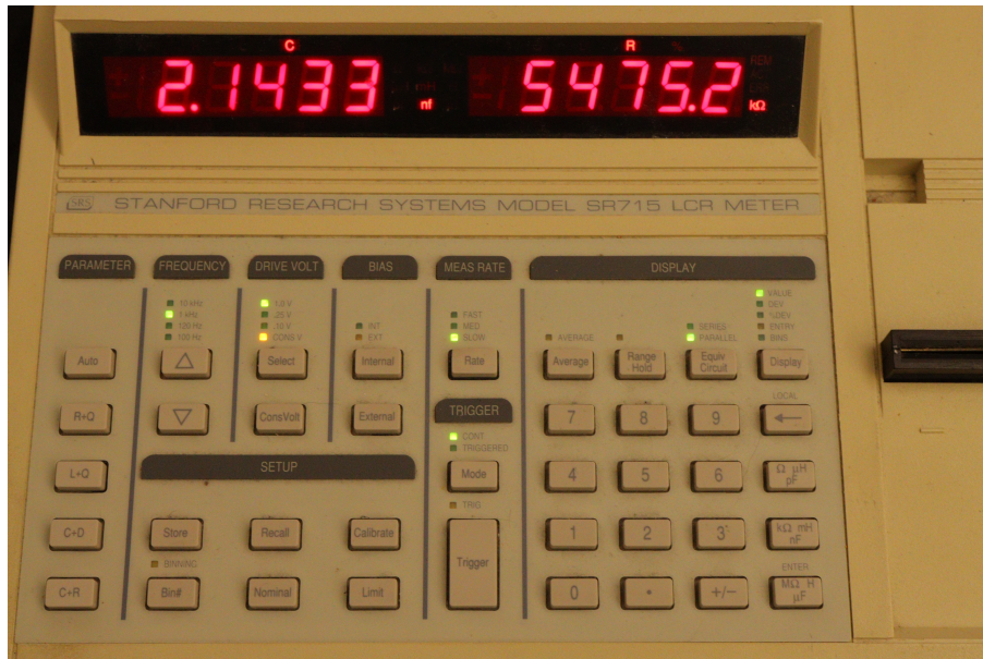
Figure 8: The front panel of the LCR measurement bridge
